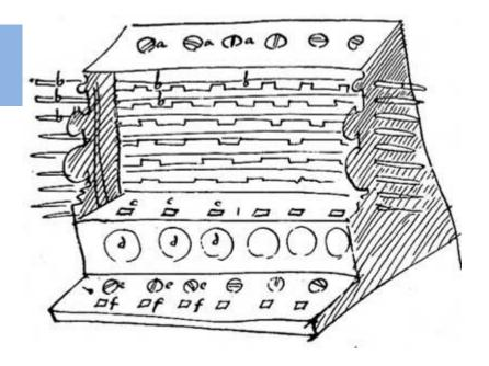
*In order the revolutions of the wheels* to be in the same direction, intermediate wheels **h** are necessary.
